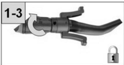
The machine is connected with a protecting joint and suction control ring, protecting the hose from being crushed by machine and maintaining the ability of dust suction [1-4];
