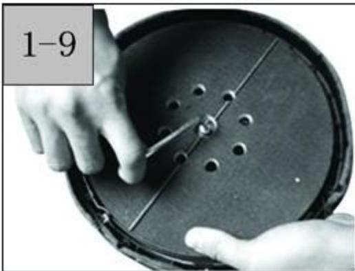
**Attention: Only install the specified velcro pad on the machine.**
